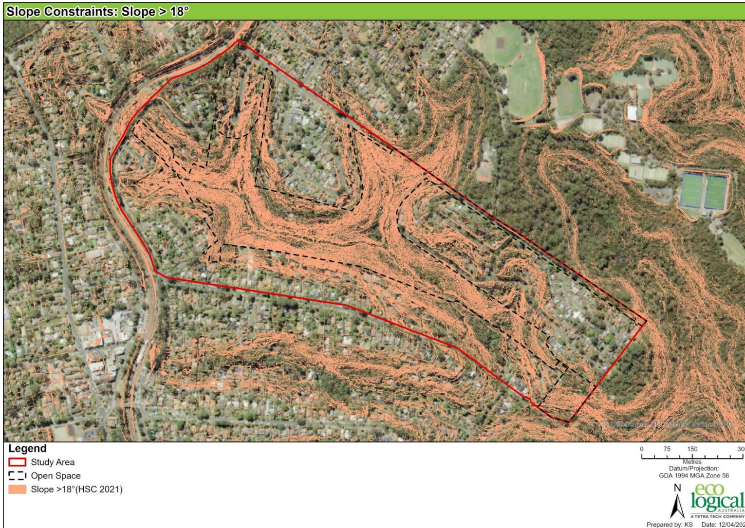
Figure 21: Slope constraints, areas >18 degrees
