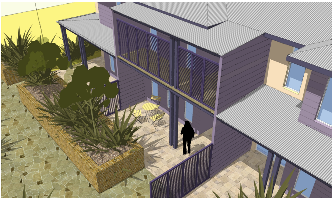
Figure 3.2(m): Fixed screens and communal planters provide privacy for ground level open spaces and rooms but allow casual surveillance of common areas from each dwelling. Adjustable screens on balconies provide for microclimate control. (E)
