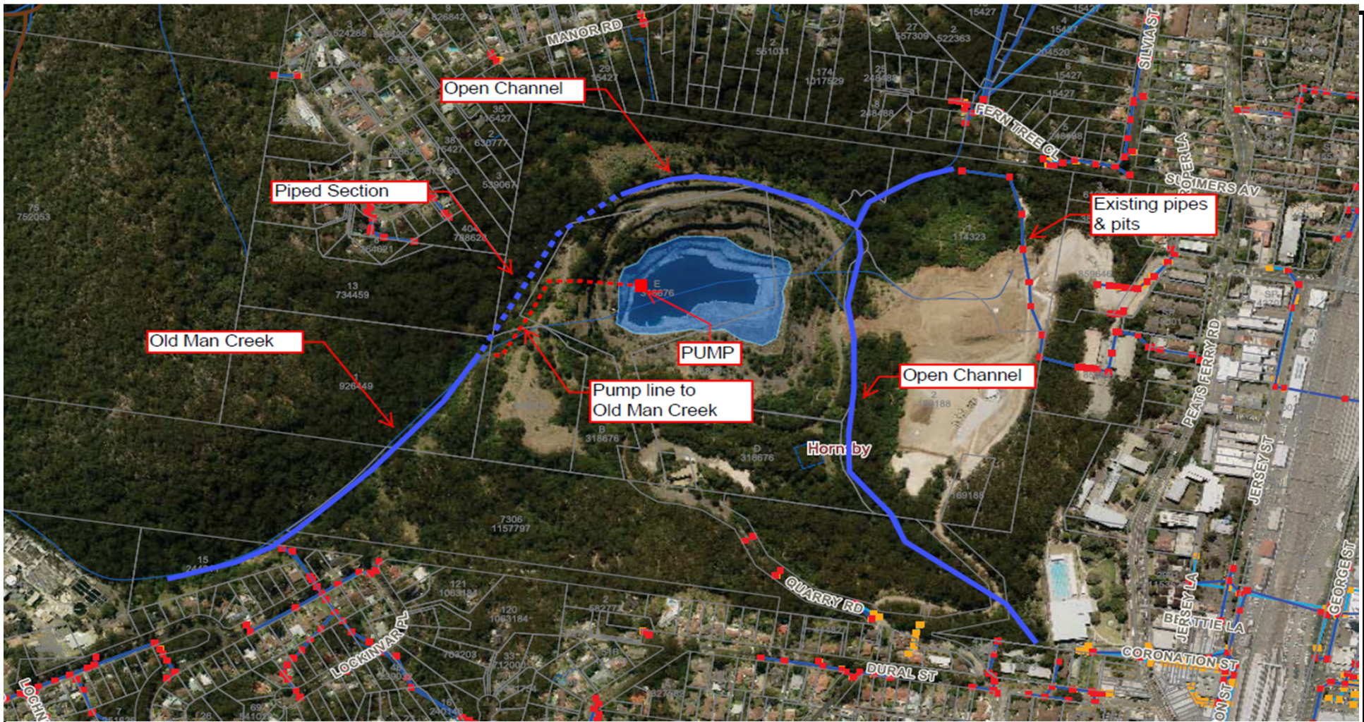
HORNSBY PARK STORMWATER DRAINAGE LAYOUT
