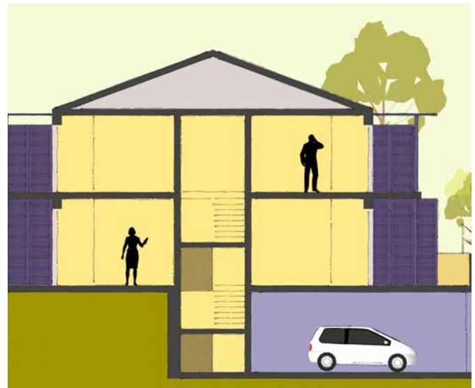
Figure 3.2(f): Building Height Controls - 2 storey town houses with a maximum roof pitch of 25 degrees and basement car parking. (E)
