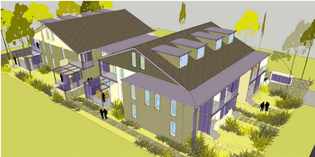
Figure 3.2(b) Residential flat buildings are an effective alternative to town houses. Positive responses to desired future character include deep soil landscaping along all site boundaries, a limit to the footprint of each building, potential for an attic storey within a gently pitched roof, dwellings that are oriented toward the front and rear boundaries and car parking that is concealed below ground level and within the building footprint.(I)
