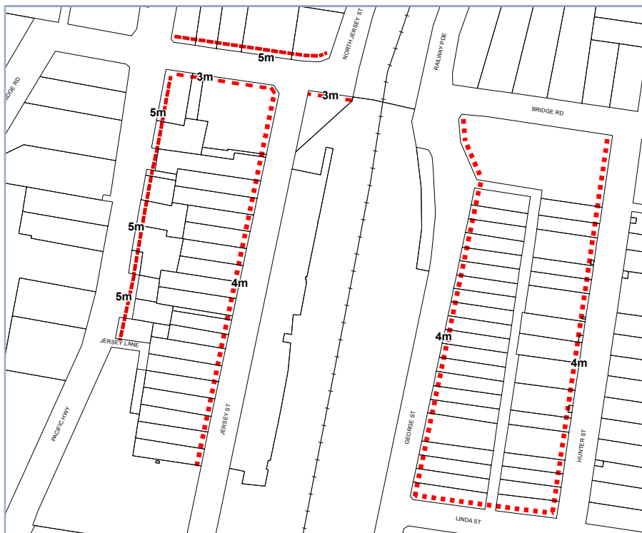
Figure 4.2(e): Hornsby (Bridge Road) Setbacks. (C)
