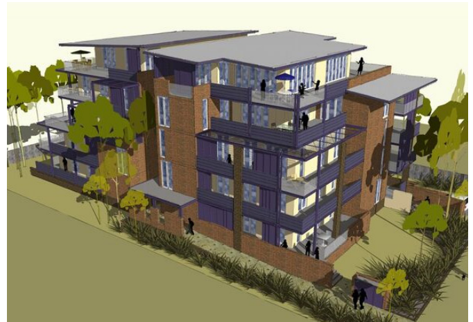
Figure 3.4(e): Building Height. (l) Height controls are based on a typical residential floor to floor height of 3 metres, with a 0.5 metre allowance for roof articulation and a 1 metre basement projection.
