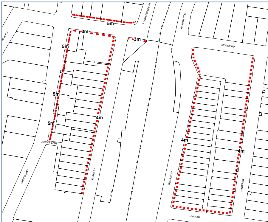
Figure 4.2(e): Hornsby (Bridge Road) Setbacks. (C)
