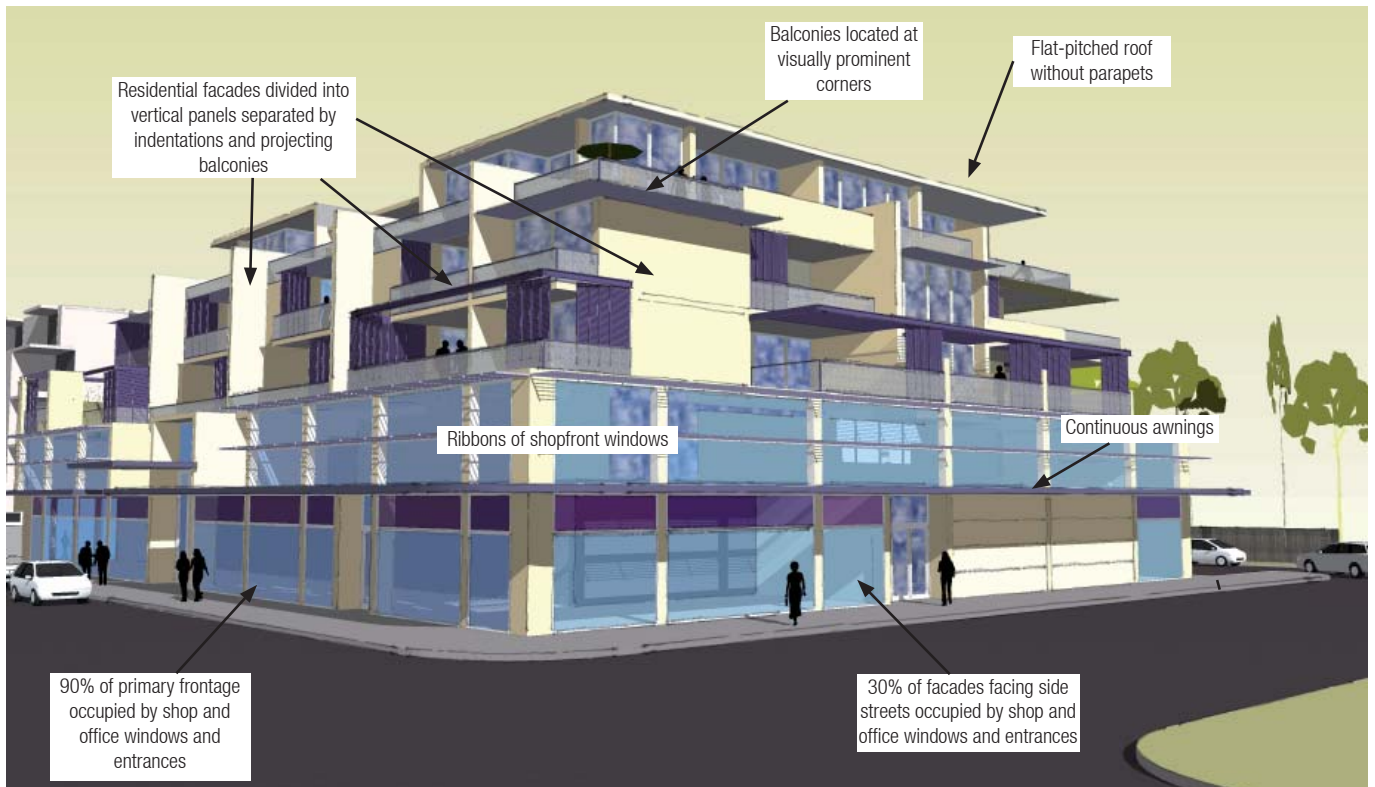
Figure 4.4(e): Articulation of facades.(E)
